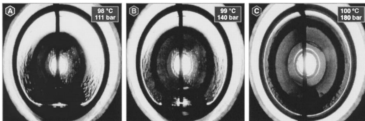
FIG. 8. Interlaced video images of the view cell under reaction conditions (5 mol% 2-octanol, 2.5 mol% O 2 -N 2 mixture, 92.5 mol% CO 2 ), showing a two-phase equilibrium of a liquid 2-octanol-rich phase and a "sc" CO 2 -rich phase at 100 °C. The amount of liquid phase decreases with increasing pressure. The vertical line is the thermocouple and at the bottom of the reactor the liquid phase is clearly visible. The round bright spot at the opposite end of the cell is the sapphire window used for illumination. In the middle of the reactor at the bottom lies the magnetic stirrer.
